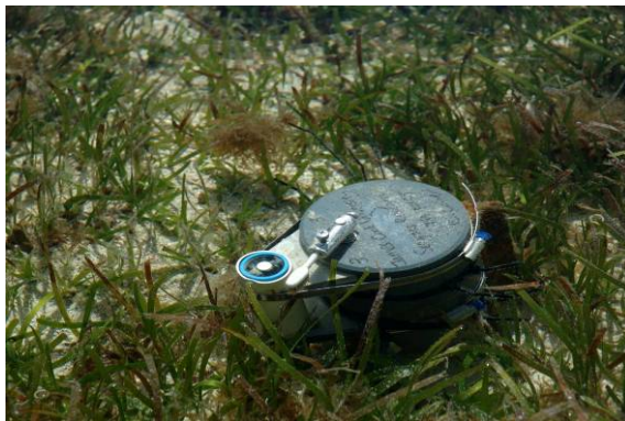
Submersible Odyssey™ photosynthetic irradiance autonomous logger deployed at Green Island.
