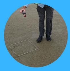
Make sure the photo details are noted on the data sheet so the photo can be matched with the quadrat details.
