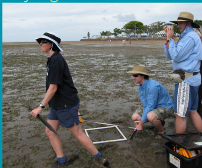
Layout and peg down the three 50m transects, parallel to each other, 25m apart & orientated perpendicular to shore (heading out to sea or deeper water)
