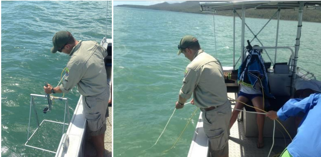
Figure Appx-2.3. Deployment of drop camera, with one operator controlling in-water frame assembly and the other operator checking images live from GoPro (note: screen operator requiring to shelter under towel to reduce screen glare).
