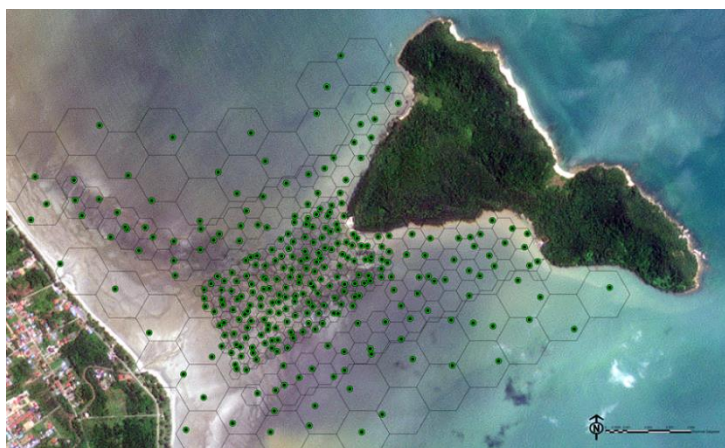
Figure 3. Field survey plan for mapping seagrass meadows between Pulau Setindan and the mainland (Mersing, Malaysia), showing 2,500m 2 , 1 ha and 5 ha tessellated hexagons with randomised points within each. Smaller hexagons cover the intertidally exposed banks, while the larger are positioned in the deeper turbid waters. Image capture 4th September 2022 [38].
